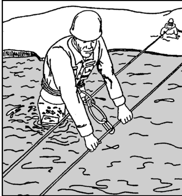
Figure 9-4. Stream crossing using a handline.
